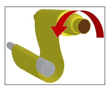
2. Position new film roll so that the film is coming off the top of the roll in a counterclockwise direction when viewed from the right side.
