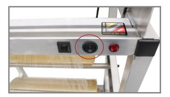
5. Turn on the machine using the on/off switch to the right front of the machine. It will take approximately 12 minutes for the film cut off rod to come up to cutting temperature.
