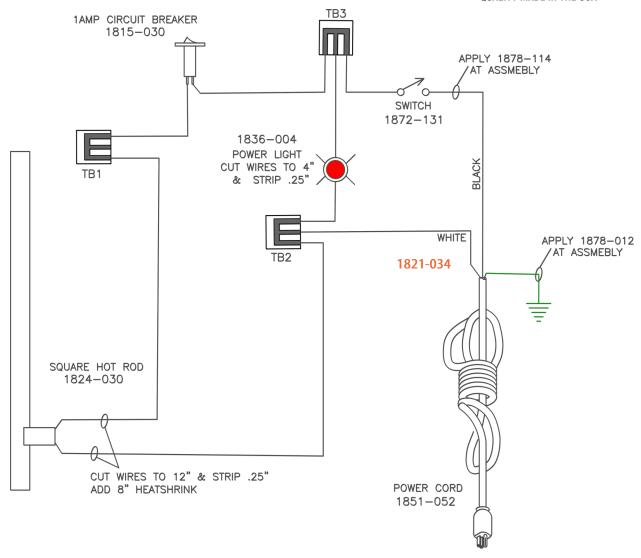
NOTE 1: CUT 6305-306-04 IN HALF THEN TO 4" LENGTH & STRIP TO .25" NOTE 2: CUT 6305-306-05 TO 4" LENGTH & STRIP TO .25"
