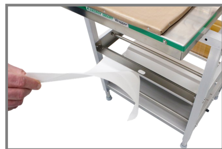
Use the tension created to pull against the cutter edge to cut the butcher paper
