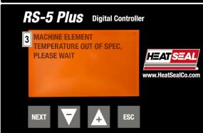
There are four (4) alarms that can occur anytime the controller is powered. The L Sealer will not operate during any of these alarm conditions. The alarms will show on the screen until the solution is fixed.
