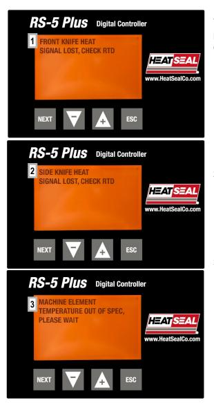
There are four (4) alarms that can occur anytime the controller is powered. The L Sealer will not operate during any of these alarm conditions. The alarms will show on the screen until the solution is fixed.
