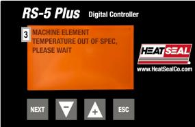
There are four (4) alarms that can occur anytime the controller is powered. The L Sealer will not operate during any of these alarm conditions. The alarms will show on the screen until the solution is fixed.
