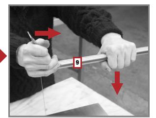
While flipping the lever into place, pressure must be exerted on the cutter arm (9) to allow the wire to be tightened securely. Force lever over slowly to tension wire. Check that wire stays centered in the slot on the flip lever.
