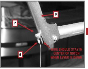
• Then place the large loop (6) over the anchor screw (7) on the flip lever (8) on the handle.
