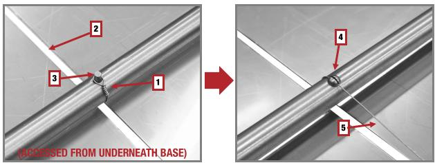
• Wire has one large loop and one small loop on the ends. Pass the wire end with the small loop (1) through the slot in the base (2), then over stud (3).
